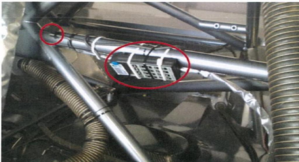
Figure 2. Noise dosimeter placement –V8 Supercar Driver 2.
